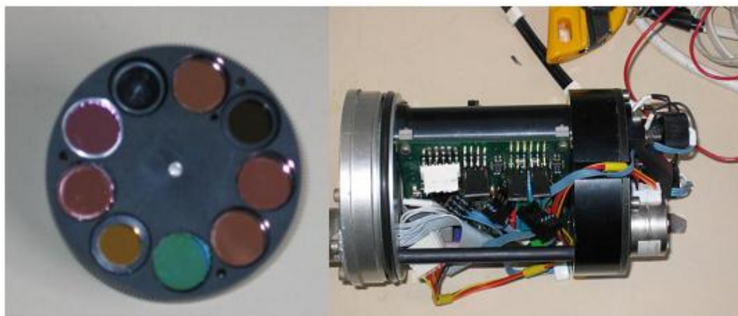
Figure 3. Filter wheel which is rotated by a motor
